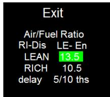
This is your lean threshold for the cutout. If you have ENABLED the lean cutout, the output will shut down if you go leaner than this setting. Pushing the control button in will turn the area grey and you can scroll up or down to the correct value. Push the control button in again to save.
