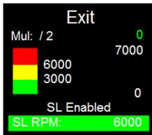
This is the Shift Light RPM. Your gauge is the shift light. The entire screen will jump to a solid color telling you it is time to shift. Pushing the control button will toggle the color to grey. Make your adjustment to up or down to fit your needs. This is the RPM point your shift light will come on. Push the button again.
