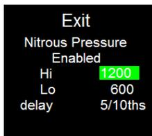
This is the HI side limit of your cutoff; the output will shut down if you exceed this pressure. Pushing the control button in will turn the area grey and now you can scroll up or down to the correct value. Push the control button in again to save.
