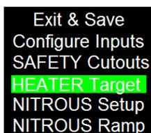
Push control button in and enter the HEATER Target screen.
