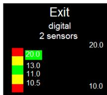
This is the HI side set point where your air fuel display will change from yellow to red. Pushing the control button in will turn the area grey and now you can scroll up or down to the correct value. Push the control button in again to save.
