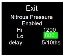
This is the Lo side limit of your cutoff; the output will shut down if you drop below this pressure. Pushing the control button in will turn the area grey and now you can scroll up or down to the correct value. Push the control button in again to save.
