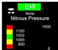
Push the control button in to save. You have programmed your PRESSURE Inputs and have returned to the INPUT main screen. Highlight Exit and push the control button in.
