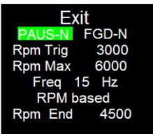
This is the ramp reset/resume option. This tells the gauge to either resume your ramp [PAUS-Y] or reset to beginning [PAUS-N]. EXAMPLE: while ramping you lift off the gas and then step back into it, you can either have the ramp continue where you left off or restart from the beginning. You can toggle the setting by pushing the control button while it is highlighted.
