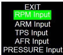
Starting from the Exit & Save menu shown above, toggle the control button down until RPM Input, is highlighted.
