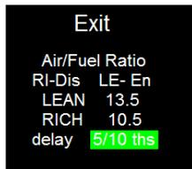
This sets the time that either the lean or rich condition must exist for before a cutout will happen. Pushing the control button in will turn the area grey and you can scroll up or down to the correct value. Push the control button in again to save. [0 – 1 sec]
