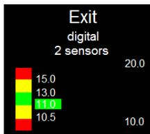
This is the low/mid side set point where your air fuel display will change from yellow to green. Pushing the control button in will turn the area grey and now you can scroll up or down to the correct value. Push the control button in again to save.
