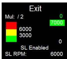
This is your HI side range for the tach. The closer you keep this number to your red line works nicely. Push the control button in and it turns to grey allowing you to make adjustments. Push the control button up or down to increase or decrease the value. When you get to the desired RPM, push the control button in to save it. This number is for the resolution of your tach scaling only, nothing more.
