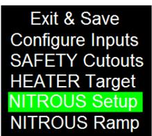
Push the control button in to enter the NITROUS Setup screen
