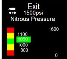
This is the mid/ hi side set point where your pressure display will change from green to yellow. Pushing the control button in will turn the area grey and now you can scroll up or down to the correct value. Push the control button in again to save.
