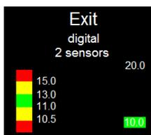
This is the low side set point for your wide-band scaling. The closer this number is to your low number the finer the scale will be. Pushing the control button in will turn the area grey and now you can scroll up or down to the correct value. Push the control button in again to save.
