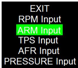
With ARM highlighted, push the control button and you will enter the ARM input menu.
