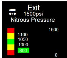
This is the low side set point where your pressure display will change from red to yellow. Pushing the control button in will turn the area grey and now you can scroll up or down to the correct value. Push the control button in again to save.
