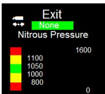
Pushing the control button in will turn the area grey and now you can scroll up or down to find the proper PSI sensor setting. Your choices are 15psi, 50psi, 100psi, 200psi, 1500psi and, 1600psi. Once you have chosen the proper sensor push the control button in to save.
