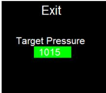
This is your target pressure for your bottle heater. The heater will turn off above this setting. It also has a safety that disables the heater if the pressure did not rise after 15 mins or if the pressure drops too low. Pushing the control button in will turn the area grey and you can scroll up or down to the correct value. Push the control button in again to save.
