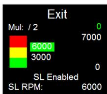
This is the HI change color. The displayed RPM will change from yellow to red above this point. Push the control button and it will turn grey and you can make your adjustments. Push the control button again to save it.
