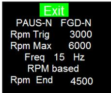
Highlight EXIT and push the control button to save and exit.
