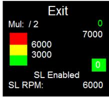
This is your LOW side range for the tach. To change this number up or down push the control button and it turns to grey allowing you to change the value. Push the control button when you get to the desired RPM. Again, this number is for the resolution of your tach scaling only, nothing more. A typical setting would be 500RPM below your idle. Push the control button to save.
