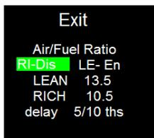
This setting enables or disables the rich side cutout only. You can toggle the setting by pushing the control button while it is highlighted.
