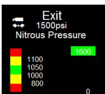
This is the HI side number used for scaling. The closer this number is to your highest number the finer the scale will be. Pushing the control button in will turn the area grey and now you can scroll up or down to the correct value. Push the control button in again to save.
