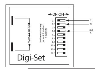
This time delay switch is set to activate a second stage of nitrous after a delay of 1.10 seconds
