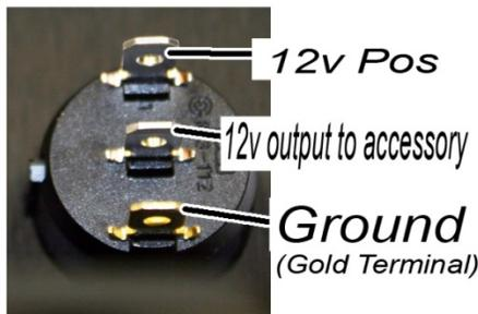
Bottle Opener Switch Wiring
