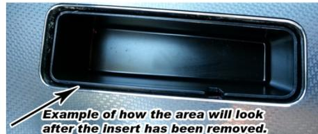
Once the coin tray is removed simply place the switch panel in place of the coin tray.
