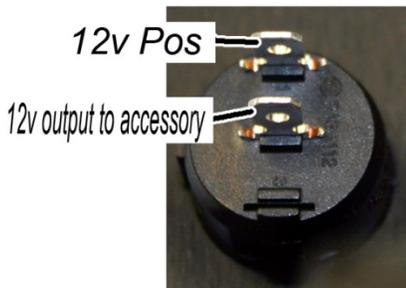
On/Off Switch Wiring
